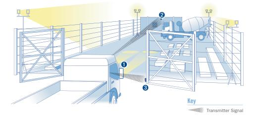
With their impressive 100m range and long battery life EasySwitch **Key Fobs** ① offer the perfect solution for long distance, reliable wireless automation. In conjunction with the ESR.4 **Receiver** ② up to four circuits can be switched from a single transmitter to operate gates ③, lights or roller shutters for example.
