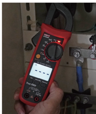
NCV multi-segment display and audio/visual alarm
